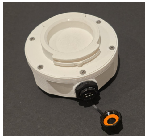
AnchorVate - USB-C charging port
